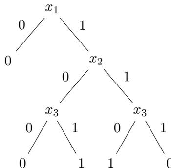
A decision tree computes a function  $f: \{0, 1\}^n \rightarrow \{0, 1\}$  in a natural way: Query the variable at the root, follow the edge labeled by its value, and continue until a leaf is reached, then output its value. The above decision tree computes the function  $x_1$  AND  $(x_2$  XOR  $x_3)$ . The following decision tree computes the same function:
