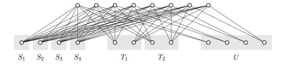
This is a graph with 8 top vertices and 12 bottom vertices, which are partitioned into 7 sets  $S_1$ ,  $S_2$ ,  $S_3$ ,  $S_4$ ,  $T_1$ ,  $T_2$ , and U. The degree of each vertex depends on the type of set it belongs to as follows:
