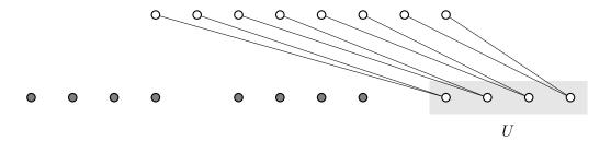
The vertices in U have now the highest degrees, so algorithm A will also include those in the cover C. The vertex cover C produced by algorithm A will therefore consist of the bottom 12 vertices. The graph, however, has a vertex cover of size 8 consisting of all the top vertices. To summarize, in this example algorithm A outputs a vertex cover that is (at least) 1.5 times larger than the smallest one. You can generalize this example to prove the following theorem:
