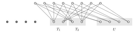
At this stage the degree of the top vertices has dropped to 3, so the next batch of vertices to be included in the cover by algorithm A will be those in  $T_1$  and  $T_2$ , resulting in the following state:
