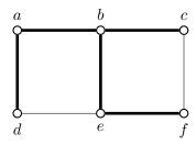
**Theorem 3.** Every connected graph has a spanning tree.
