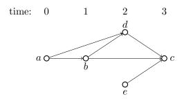
In general, a parallel schedule of a DAG G is a partition of the vertices of G into sets  $V_0, V_1, \ldots, V_\ell$  such for every edge (u, v), if u is in  $V_i$  and v is in  $V_j$  then i < j. The number  $\ell$  is the duration of the schedule.
